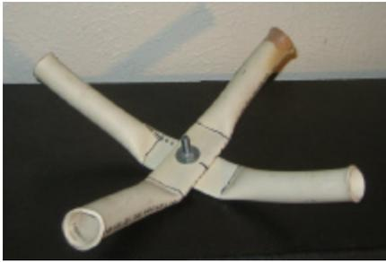
The tricky part was to create a top joint which would bring the four side poles of the pyramid together with the four corner ropes.
