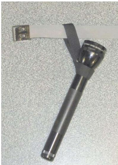
You can slip the top portion of the strap under your belt and fold it over, closing the snap and forming a belt loop. The snap lets you put on and take off the tool strap without removing your belt. It works fine with trouser belts or any kind of tool belt. Slip it between your cell phone and swiss army knife, or maybe next to your batarang.
